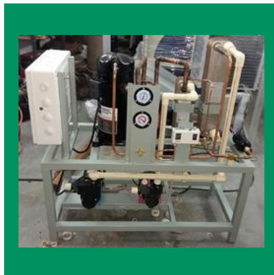
Water Cool Chiller
